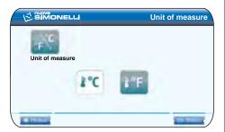
Use the rotary switch to select and press it to confirm.
