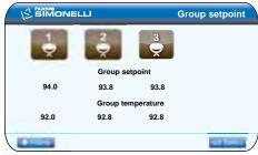
Use the rotary switch to select the coffee group to adjust and confirm by pressing.
