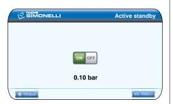
**ON 0.50 bar**: during the OFF state, the machine maintains a pressure of 0.50 bar and the display (set to minimum brightness) reads "LOW CONSUMPTION.
