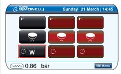
Once the washing has been finished, the rinse stage is requested automatically:
