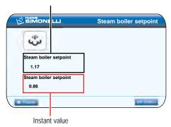
Turn the rotary switch to select the required pressure / temperature for the boiler (see the table on the following page) and then press the switch to confirm the setting.
