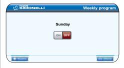
To save changes, press the rotary switch. At this point, the day is active, the hours will start to flash for the ON time.
