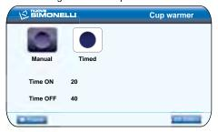
Use the rotary switch to edit the ON and OFF times and then press to confirm.
