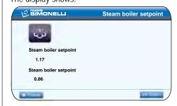
Select the steam icon and confirm with the rotary switch.
