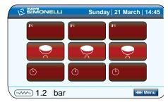
Press the button on and coffee key together in case of the S version, or the long coffee key on the V version; the corresponding group will be disabled, causing the display to read (E.g. group 1 de-activated):
