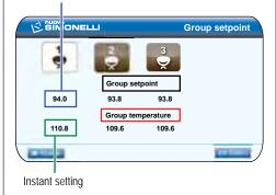
Turn the rotary switch to select the required temperature for the group, then press to confirm.
