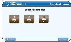
Select the coffee unit to apply the "standard dose" settings and press the rotary switch to confirm.
