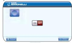
Selecting ACTIVE or off it is then necessary to use the rotary switch to set the hours and minutes after which the alarm message appears. After the minutes have been set, the machine returns to the main menu.
