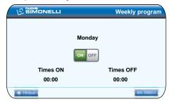
To change the configuration for one day, this day must be shown on the display and then the rotary switch must be pressed.
