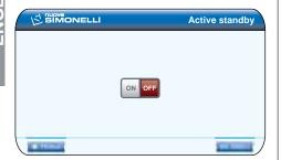
ON 0.10 bar: during the OFF state, the machine maintains a pressure of 0.10 bar and the display (set to minimum brightness) reads "LOW CONSUMPTION".
