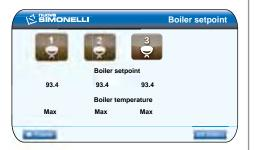
Select the coffee boiler to be adjusted and confirm by pressing the rotary switch.
