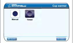
To work in "timer" mode, select the timer icon Timed (Timed) with the rotary switch and press it. The following screen will open:
