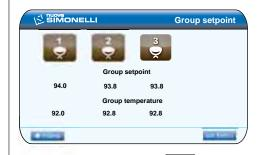
Hold down the washing key to access offset and group temperature adjustment. The next screen will be:
