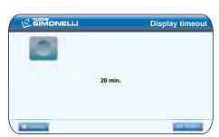
Use the rotary switch to choose the time (minutes) and press to confirm.
